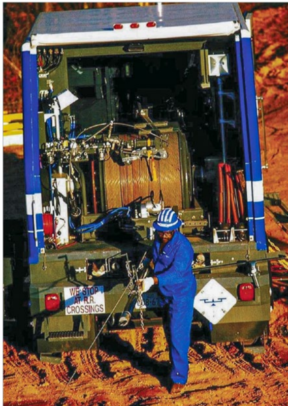
Fig. 15 —A Maxis Express logging truck. At center, the large cable drum with one end of the cable leading into a well (courtesy of Schlumberger).
