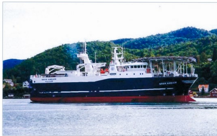
Fig. 14 —GECO Angler, a seismic vessel, here pictured in 1998 during its maiden journey in Aalesund, Norway. At the stern, it could tow seismic streamers; at the bow, one can clearly see the helicopter landing deck (courtesy of Schlumberger).
